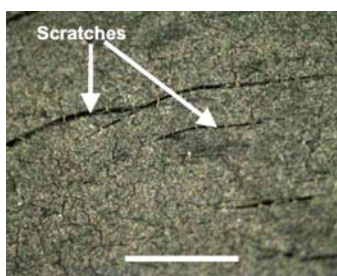
Figure 6: Cracks in sample surface prior to RBBT
