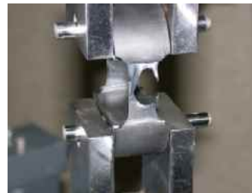
Figure 2: Failure occurred in the cut section
